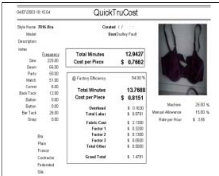
Screen above: This screen shows the data input for total sewing length and the nine (9) other categories or factors.
